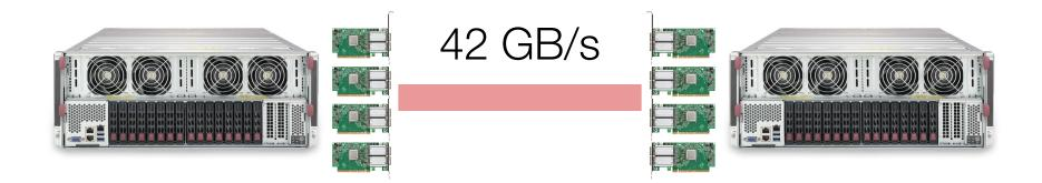
The GPU RDMA (Remote Direct Memory Access) capabilities of the InfiniBand cards and the V100 GPUs allows for a inter-node memory bandwidth of 42 GB/s. 84% of the 50 GB/s theoretical peak allowed by the four cards. 50 GB / s = 4 cards \* 100 Gb/s / (8 bits/byte)
