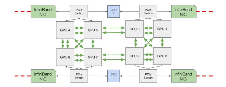
Each GPU has six NVLink connections which allows for four non-overlapping pathways to be drawn through all eight GPUs on the system and out an InfiniBand card, optimizing both GPU to GPU and node to node communication during distributed all-reduce. (See Sylvain Jeaugey's "NCCL 2.0" presentation for more information.)
