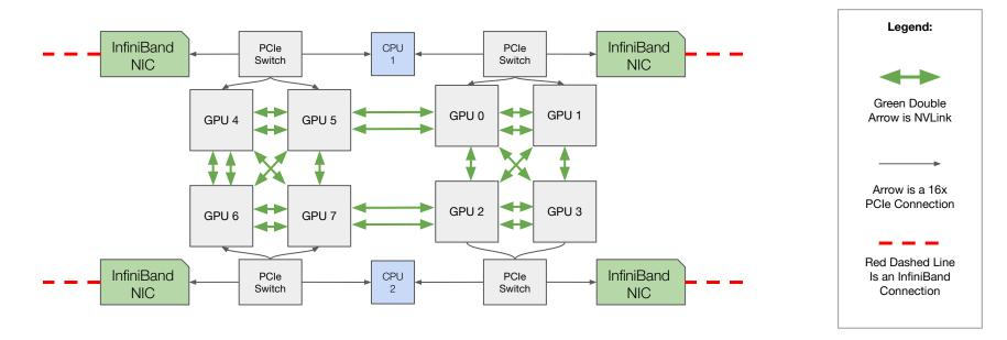
Four InfiniBand NICs are placed alongside the NVLink fabric underneath a PCIe switch. They are used for GPU RDMA during the distributed all-reduce operation.
